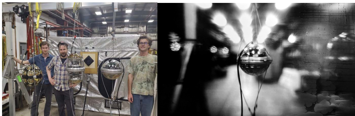
Figure 7: (Left) Artist Duke in the center with his two student assistants. The silver cube behind them is the camera body; the ice lens is behind the black diamond. (Right) An image of an IceCube digital optical module taken with an ice lens.
